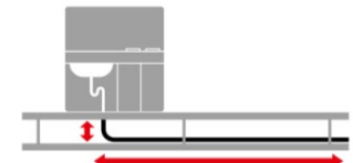
Bridgestone's "Smart Siphon" enables drainage system adaptable, creating more underfloor space and plumbing distance.
