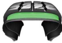
Module 2 Belt (reinforces tire)
