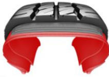
Module 1 Carcass (tire skeleton)
