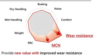
(+50% vs. Bridgestone's conventional product), an issue for EVs and increased renewable & recycled material ratio of 50%
