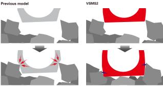
More vertical shape is less likely to catch stones, especially when the vehicle is backing, reducing risk of sidewall cut.
